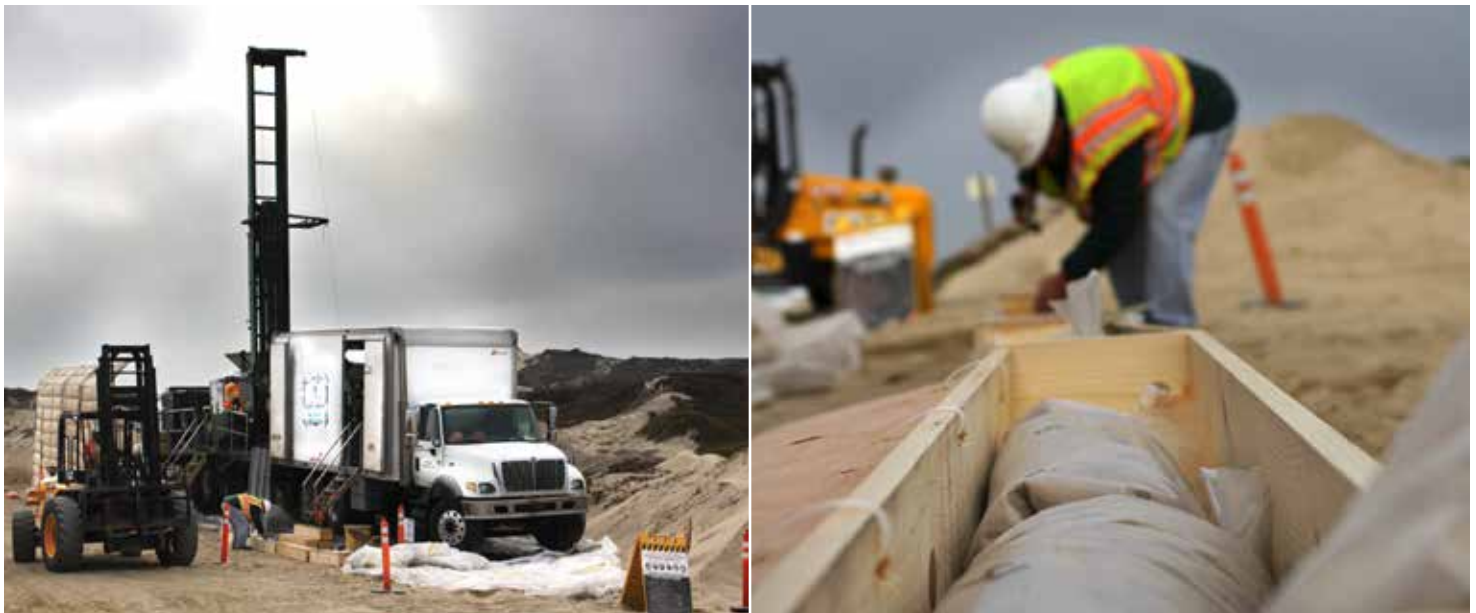
Borehole samples were drilled along the Monterey coast. The samples provide critical data needed for environmental and technical review.
